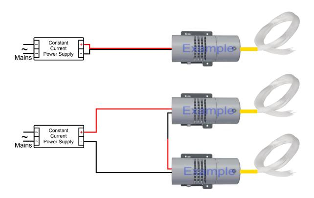
LED-18WW can be connected only with serial wiring. LED-18WW may be connected to driver. Above connection is examples and may be different from the actual.
